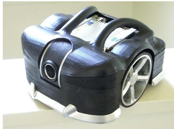
Figure 13. Fabricated robot for home monitoring
