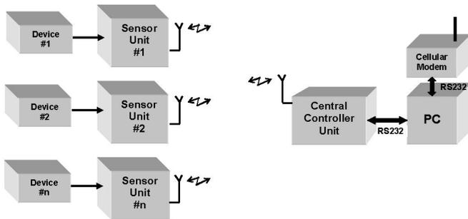
Figure 2. Functional block diagram of the system hardware
