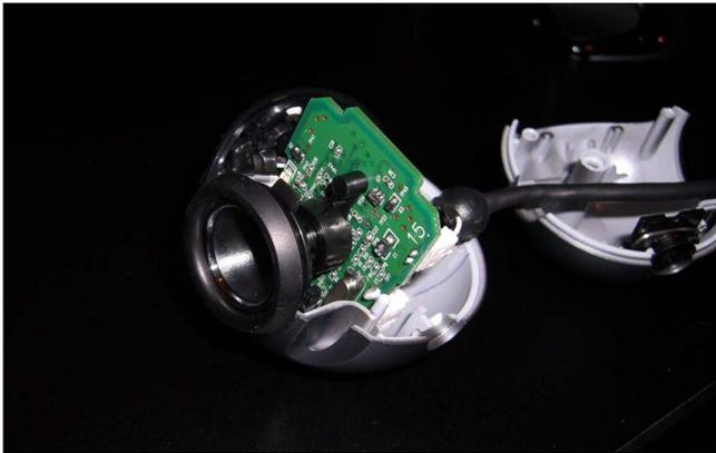
Figure 15. The camera and associated circuit of the robot for vision
